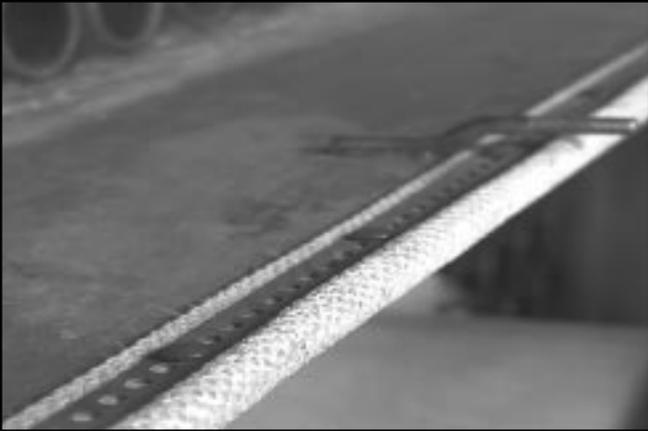
**Figure 8-27: Second to Third Pass Baffle and Gasket**
