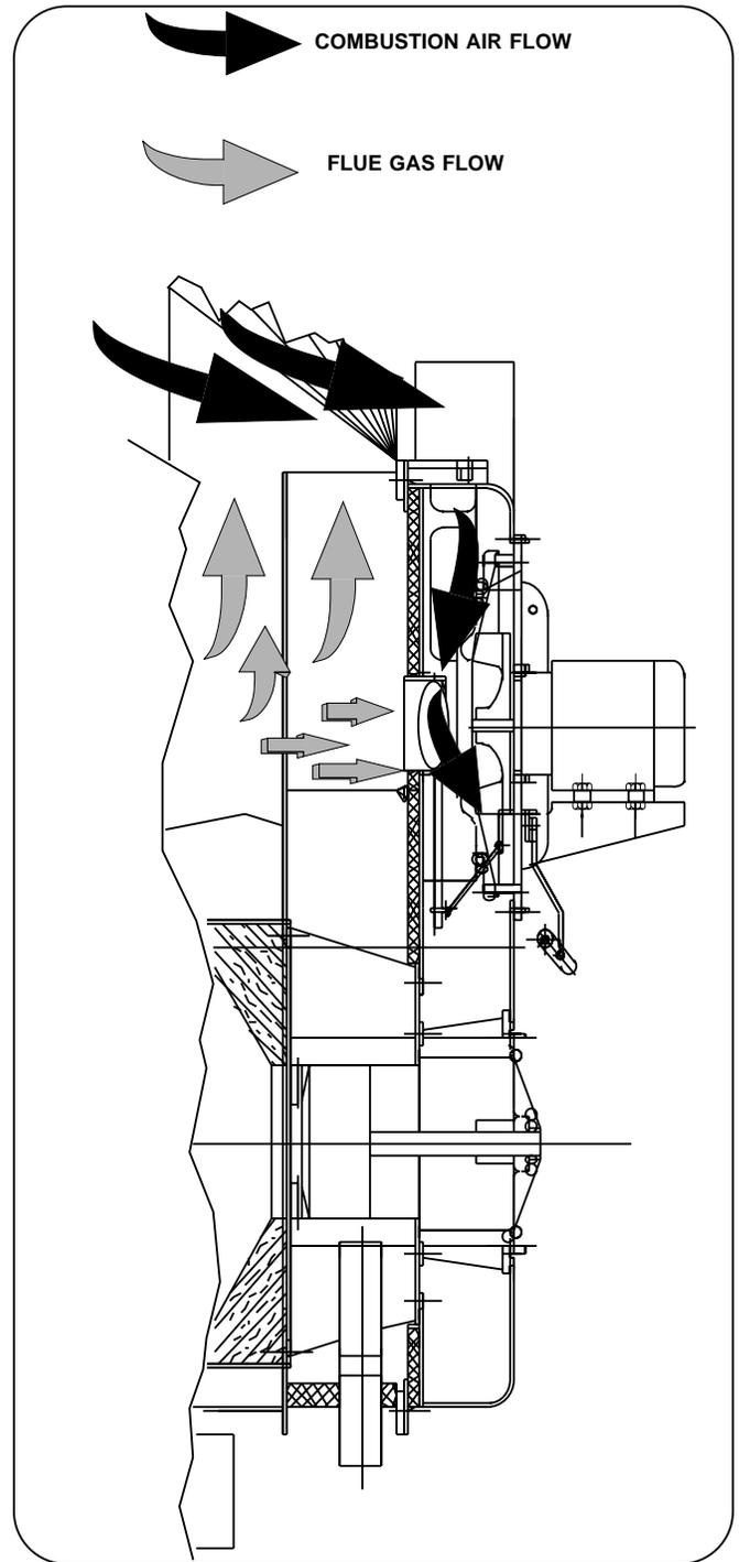
Figure 8-6: CB-LE Combustion Air and Flue Gas Flow
