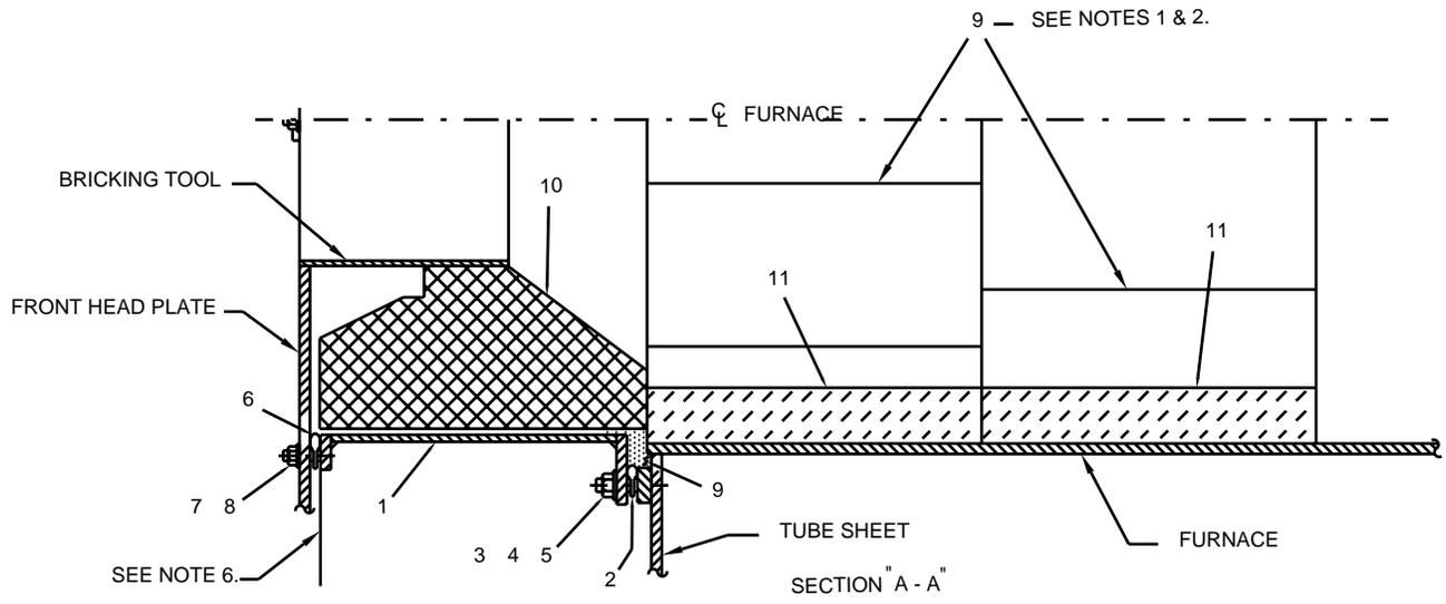
**Furnace Liner & Bricking Model CB and CB-LE**
