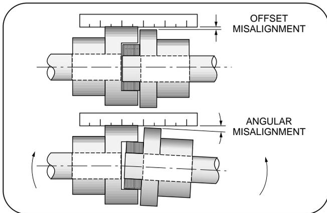
**Figure 8-21: Coupling Alignment**
