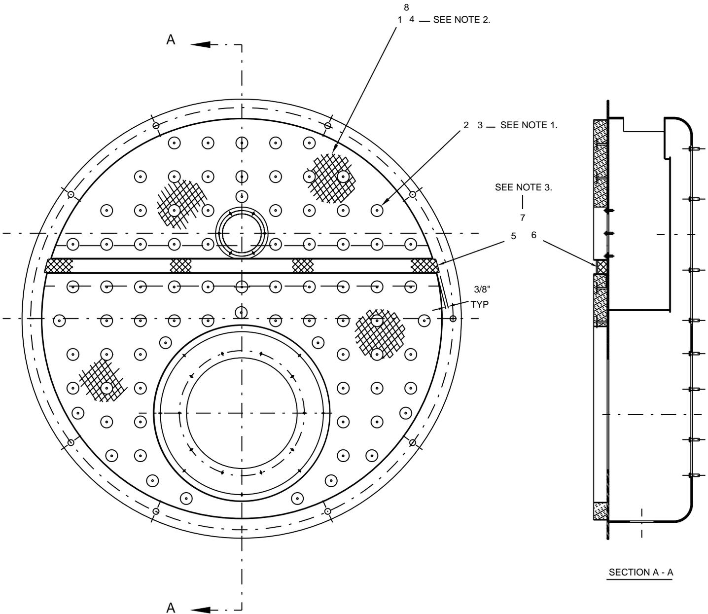
Insulated Front Head Inner Door - Model CB-LE
