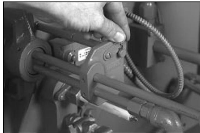
Figure 6-18 Oil Gun Locked Out
