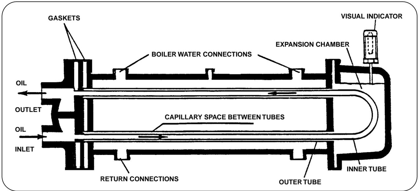
Figure 8-39: Circuit Layout of Hot Water Oil Heater
