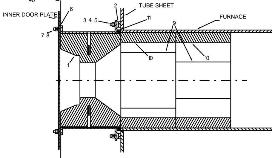
Figure 8-26: Dry Oven and Furnace Liner Tile
