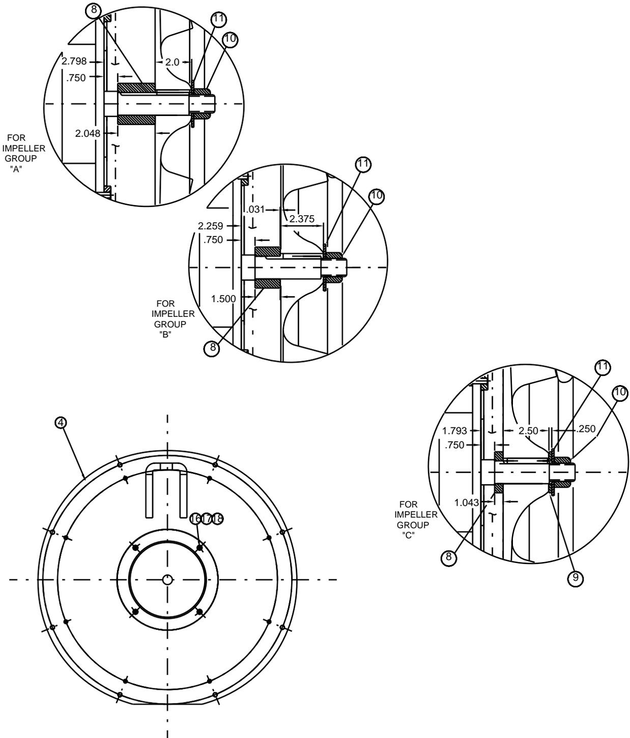
Figure 8-14: Blower Cartridge Assembly
