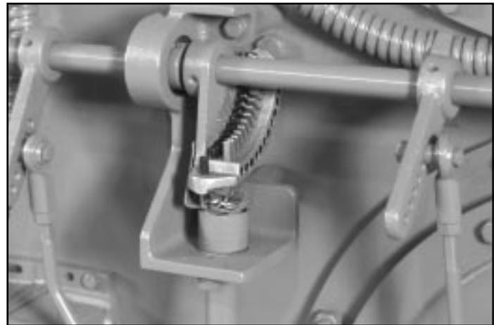
**Figure: 2-13 Gas Modulating Cam**
